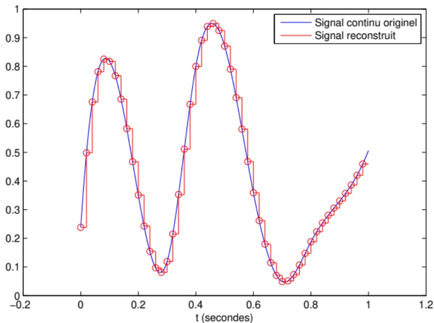
$F_e = 50$  Hz,  $T_e = 0.02$  secondes. Reconstruction encore imparfaite.
